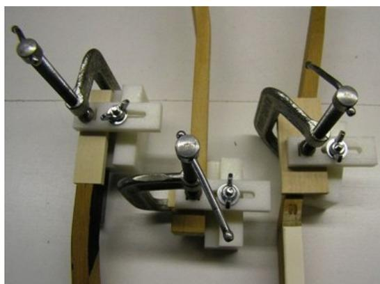
Figure 4. The new button and mortises have been put onto the caul portion of the fixture, the base of the fixture has been centered between the lines drawn earlier, then glued and clamped.
