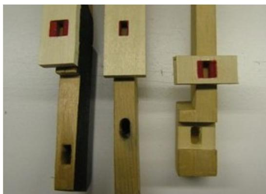
Figure 3. The damaged button and mortises have been located and removed, making way for the new ones.
