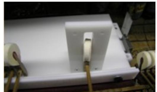
A Hammer Square employed on a Virtual Keybed to test a hammer's squareness at "strike".
