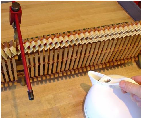
Damper return noise is annoying and replacing damper felt expensive. I have had good luck employing steam as an alternative solution.
